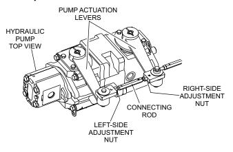
Figure 29. Pump Adjustment Components
